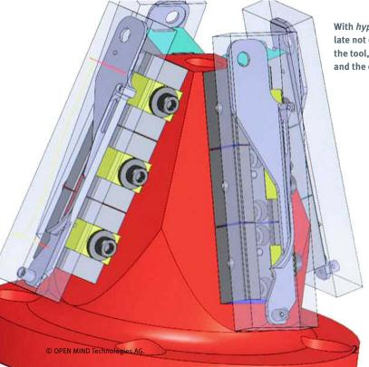
With hyperMILL® you're able to simulate not only the part in its fixture, but the tool, the tool holder, the spindle and the entire machine envelope.
